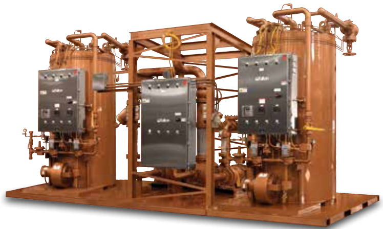
This system includes two FT-0600-C thermal fluid heaters skid mounted with three circulating pumps (one pump acts as a backup for either heater), and one FT-5000-L expansion tank (not shown). These heaters are used to provide process heat for the manufacture of asphalt roofing shingles.
