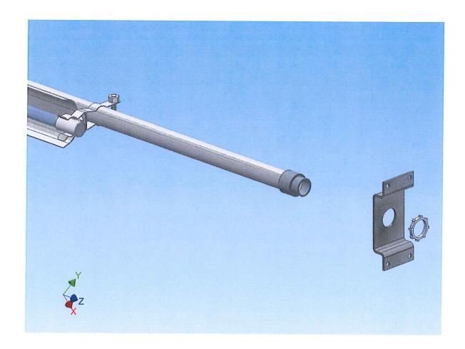
Measure the available plenum height or width as a reference and cut the tubing to size allowing approximately 1.5" on each end if using the AUV provided connectors and brackets. These tube members can be mounted horizontal or vertical, with the UVC lamps typically always mounted in the horizontal position. Refer to above figures shown on page 5, if need be, for tube and bracket mounting arrangements for both vertical and horizontal tube mounting arrangements.
