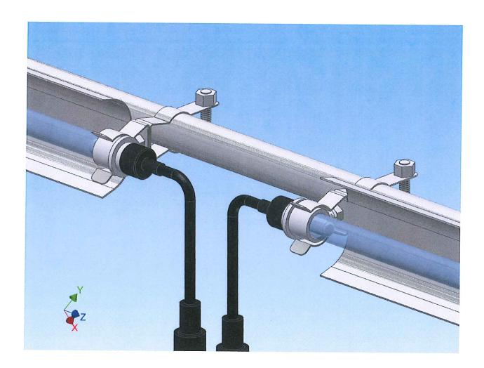
UVC lamps are provided with sure-seal moisture proof connectors on the power end of the lamp. Additionally, Lamp power cords can be provided in 8', 12', or 30' foot lengths for connecting each UVC lamp to the ballast control enclosure. Each lamp power cord has a mating sure seal connector to plug into the UVC lamp. Cord grips are provided with each lamp power cord for securing the power cord into the ballast control enclosure.
